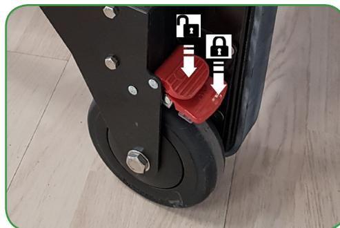
FIGURA 13 - FRENOS RUEDAS TRASERAS
